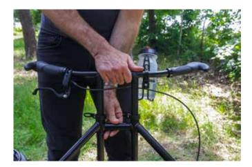
**4.** Loosen the handlebar quick-release levers to adjust the handlebar to the correct height.
