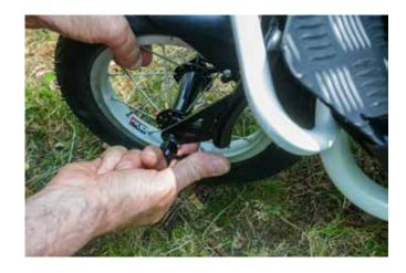
17. Then tighten it using the quick-release lever.
