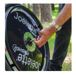
**9.** Insert the ball spindles until they lock (check that they lock by pulling on the wheel).
