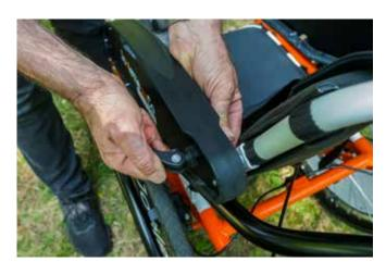
**15.** Tilt the quick-release lever once you have chosen the backrest angle.
