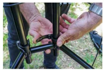
**5.** Retighten the quick-release levers.
