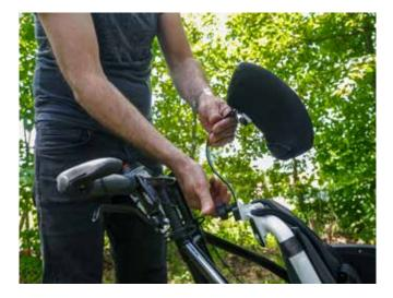
**4.** Tighten the knob to secure the headrest.
