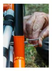
**3.** Remove the two safety pins. Then insert the two handlebar arms into the sockets provided on the chassis. Finally, replace the safety pins.
