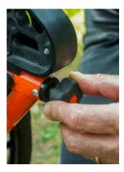
**12.** Lock each armrest by tightening the knobs.
