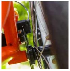
**8.** Insert the disc of each wheel between the brake pads.
