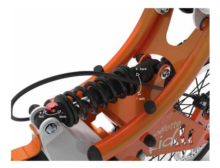
You can adjust the hardness of the shock absorber of your Joëlette Kid thanks to the nut located at the back of the spring, but also its speed of rebound with the roller on the front part.
