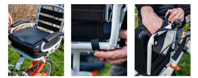
**8.** Place the cushions on the seat. Attach the snap fasteners of the straps to the back of the seat on the frame of the Joëlette Kid. Fix the backrest cushion by running the fabric lining behind the backrest and fasten the velcro.
