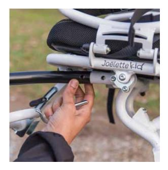
**1.** Insert the arm on the tube provided for this purpose under the seat.
