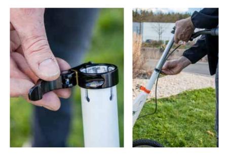
**2.** Unlock the handle clamp and insert the handlebar into the stem, then lock the clamp.
