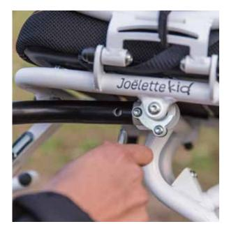
**2.** Align the holes in both tubes to put the security pin.
