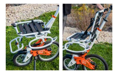
**6.** Fold the armrests on the sides of the seat and straighten the backrest.
