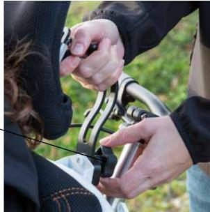
**1.** Insert the headrest support between the backrest and the plastic part and secure it using the roller.
