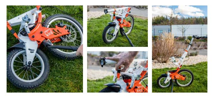
**1.** Unfold the kickstand. Position the chassis on its wheels. Detach the strap at the front, then straighten the stem until you hear the «click». Check that the frame is properly locked.
