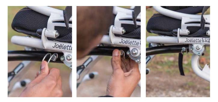
**3.** Insert the security pin and fold the rounded metal part over the tube to secure the fastener. Check that the arms are securely fixed.
