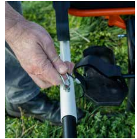
14. Lock the arms with the safety pin.
