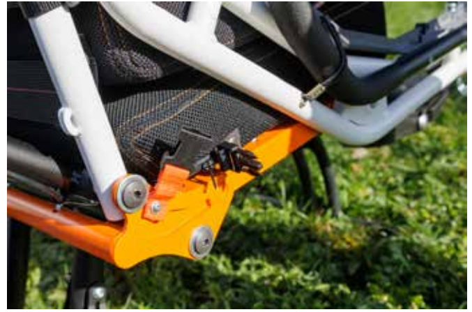
12. Fasten the side buckles sewn into the seat and fold the front panel down.
