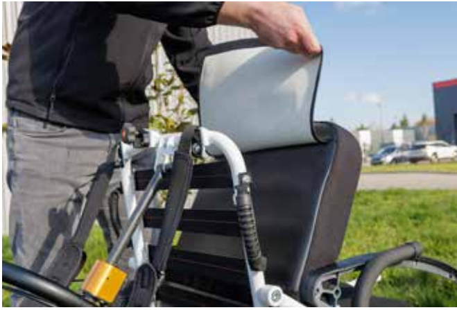
11. Pass the backrest flap behind the elastic straps and secure it with the Velcro strap.
