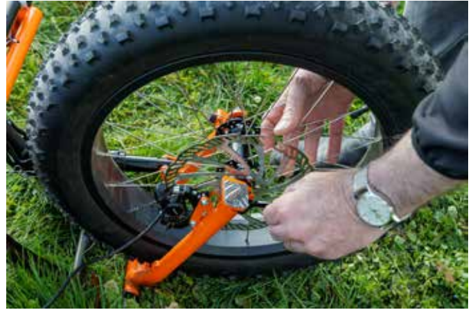
7. Position the wheel between the forks of the swingarm and secure it with the quick release.
